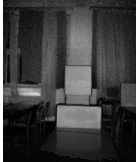
Fig. 3. Image in Figure 1 after distance-based correction without prior filtering.
