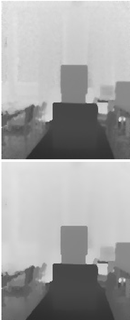
Fig. 4. Distance image before (top) and after (down) adaptive-neighborhood filtering.
