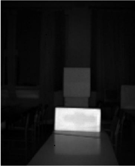
Fig. 1. A typical amplitude image delivered by a ToF camera.
